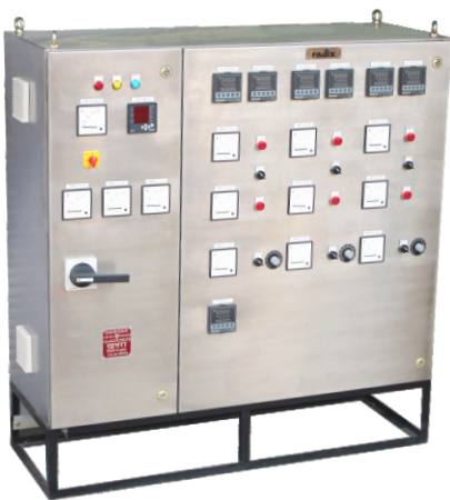
3-phase, 3-zone, SCR heating control panel in stainless steel Type of load : Resistive heater Capacity : 90kw Application : Rotary kiln
