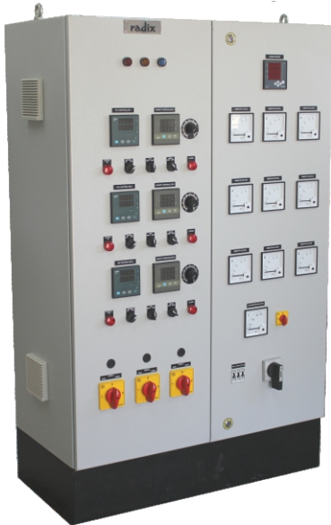
3-phase, 3-zone, SCR heating control panel with bypass facility Type of load : Transformer (primary) Capacity : 270kva Application : SS wiring drawing annealing furnace
